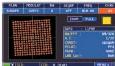
DVB-T2 rotated Constellation 256 QAM mod., on the right relative modulation parameters & M-PLP
